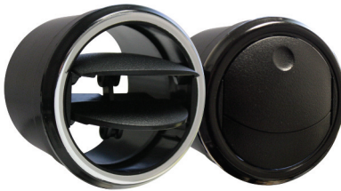
499194 Adjustable Double Vane Louver. Chrome bezel thru-dash mount. 2.706" diameter. 499193 Adjustable Double Vane Louver. Black bezel thru-dash mount. 2.706" diameter. Note: Louver Open, Close & Rotate 360°
